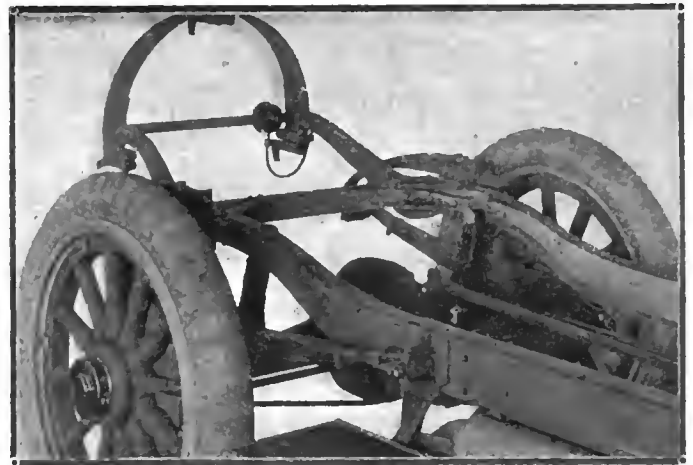
Fig. 2—Rear of the Howard chassis, showing the method of carrying the tire bracket. The spring suspension may also be seen, as well as the manner of covering the bolts on the rear hub caps
